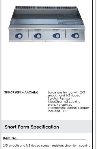
surface. 33 kW gas powered burners with thermostatic valve and self stabilizing flame. Temperature range up to 270°C. To be installed on open base installations, bridging supports or cantilever systems. Removable drawers below the cooking surface for the collection of grease and fat. Body and work top of unit entirely in stainless steel with Scotch Brite finish. Extra strength work top in heavy duty 2 mm stainless steel. Rightangled side edges to allow flush-fitting junction between units.
